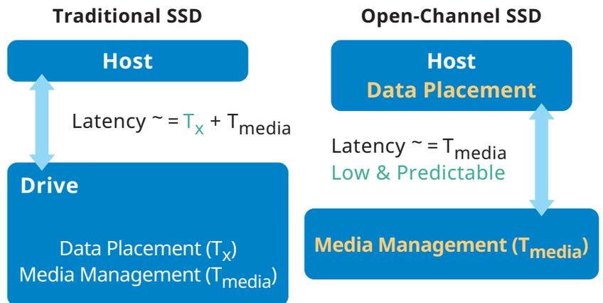
Fig. 3: in an Open Channel architecture, the SSD media's contribution to latency is transparent to the host and entirely predictable
